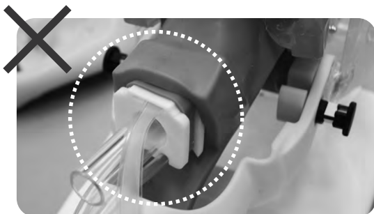
Example of inappropriate installation of tongue component
